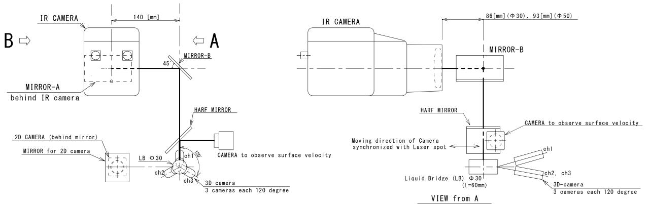
(VIEW from cooling disk side to heating disk side)
